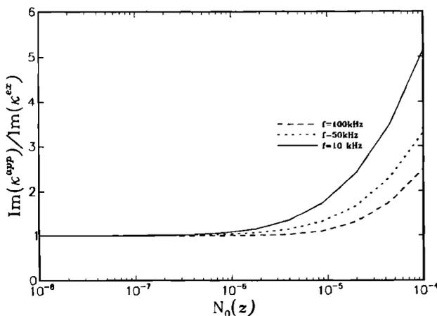
FIG. 12. Ratio of the imaginary part of the mixture wave number according to the binomial expansion (25) to the exact value given by (2) as a function of the parameter  $N_0$  appearing in Eq. (42). These results are for the same bubble spectrum used in the previous figure. The corresponding volume fraction is given by  $52.8 N_0$ , approximately.
