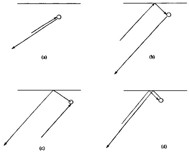
FIG. 3. The four paths by which a bubble can cause backscattering in the ray approximation of Sec. IV.
