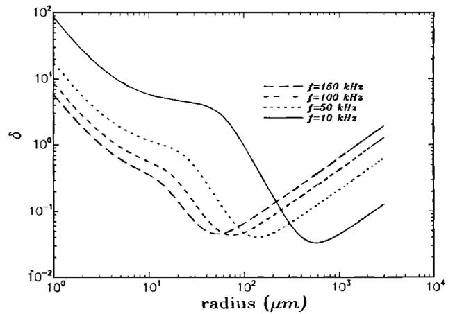
FIG. 1. The logarithmic decrement  $\delta = 2b/\omega$  as a function of the bubble equilibrium radius  $a$  for several sound frequencies  $f = \omega/2\pi$ . For each frequency the resonant radius is near the minimum of the curve.
