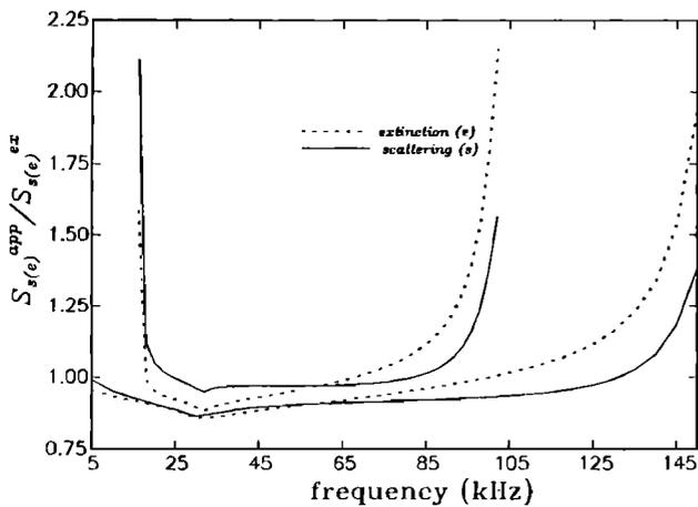
FIG. 11. Ratio of the approximations (40) and (41) to the exact results as a function of the sound frequency for two different ranges of radial integration,  $20 \mu\text{m} \leq a \leq 1.2 \text{ mm}$ , and  $30 \mu\text{m} \leq a \leq 200 \mu\text{m}$ . The bubble spectrum is the power law (42) with  $n=4$  up to  $a=100 \mu\text{m}$ , and  $n=3$  above.
