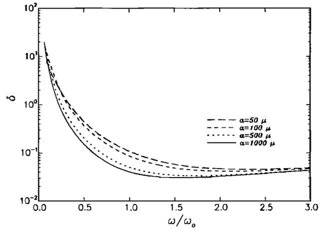
FIG. 5. Logarithmic decrement  $\delta$  as a function of the ratio of the sound frequency to the bubble resonance frequency  $\omega_0$  for four different bubble radii.
