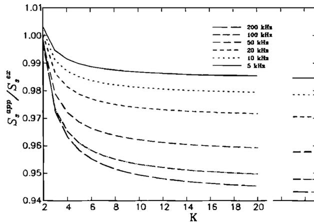
FIG. 9. Saturation effect of the ratio between the approximate and exact scattering cross sections as a function of the width of the radial integration. The parameter  $K$  is defined in Eq. (43).
